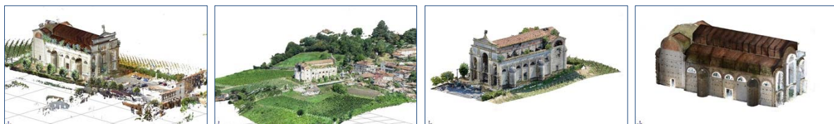
Fig. 6: Points Clouds resulting from survey operations with laser scanner and photogrammetric techniques.
